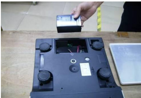
4. Disconnect the wire connection then remove the rechargeable battery.
