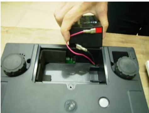
5.Prepare for a new rechargeable battery and make sure the red end connected to red wired and black end connected to black wire.
